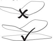
Do not scratch the image plates. Do not subject the image plates to pressure from hard or pointed objects.
