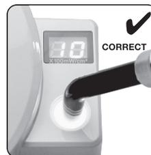
Light guide held flat and fitting exactly on the light sensor. Unit will display correct results.
