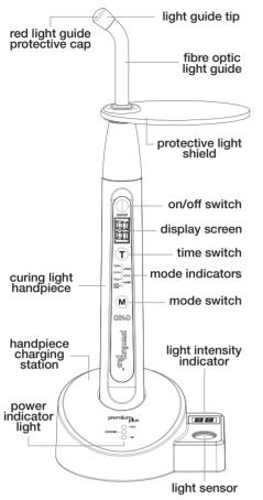
Intended use:- This curing light is intended for use by trained dental professionals only for the purpose of light curing dental resins and composites
